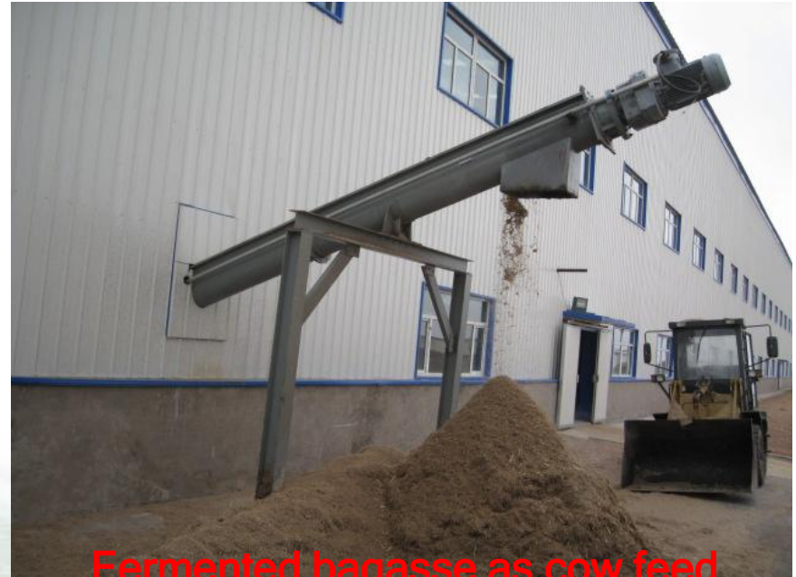
3.6X55m continuous solid state fermentor with the capacity of 8 ton ethanol/day
